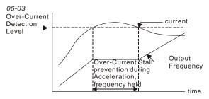
actual acceleration time when over-current stall prevention is enabled
