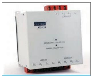
ATS models monitor all three phases continuously and give priority to DG in case any of the EB phases are unhealthy, acting as a mains single-phasing preventer (when DG is on).
