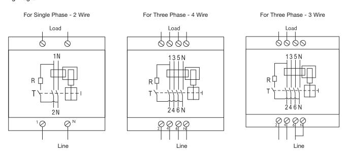
The Havells range of four pole RCCBs can be used to provide residual current protection in 3 phase, 3 wire circuits (no neutral), however a link from the neutral to an incoming should be made on the supply side of the RCCB, to enable the operation of the RCCB.
