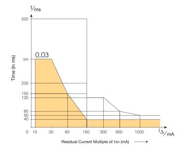
The 100 mA RCCB protects against leakage currents and indirect contact with earth loop impedance up to 500 Ohm.
