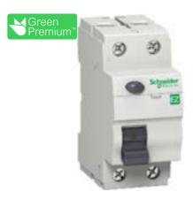
Easy9 Residual Current Circuit Breaker - 2P - 40A - 30mA - AC type - 240V
